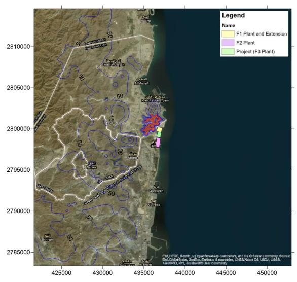
Figure B.13: Scenario 4 - Maximum 1 hour SO<sub>2</sub> (µg/m<sup>3</sup>)
