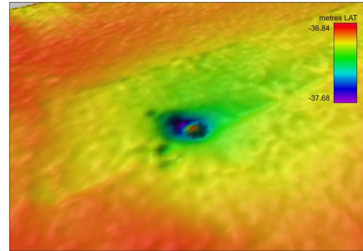
Multibeam echosounder image of ferrous debris field **7482**, looking north (x1 vertical exaggeration)
