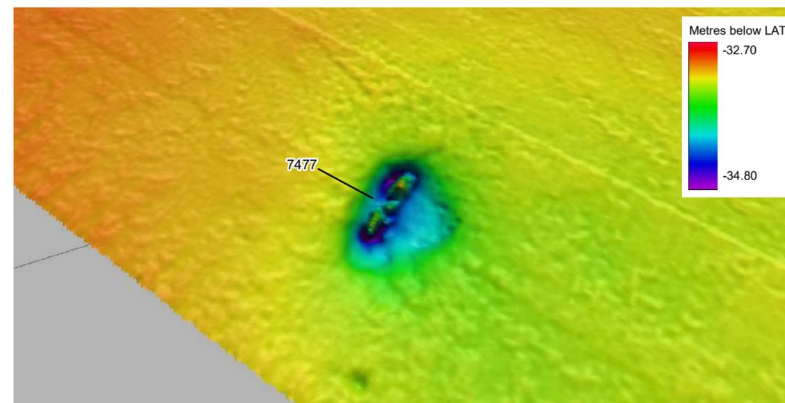
Multibeam echosounder image of wreck 7477, looking north west (x1 vertical exaggeration)
