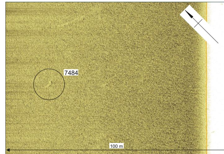
Sidescan sonar waterfall image of debris **7484**, 13.1 x 3.9 x 0.2 m
