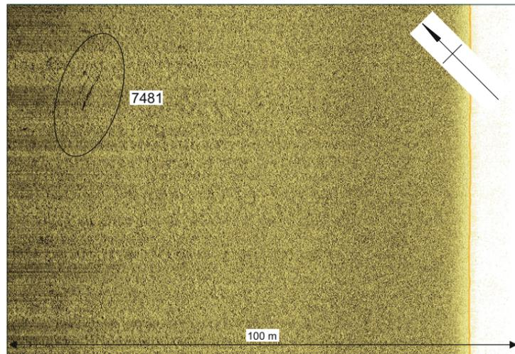
Sidescan sonar waterfall image of dark reflector **7481**, 27.9 x 0.9 m
