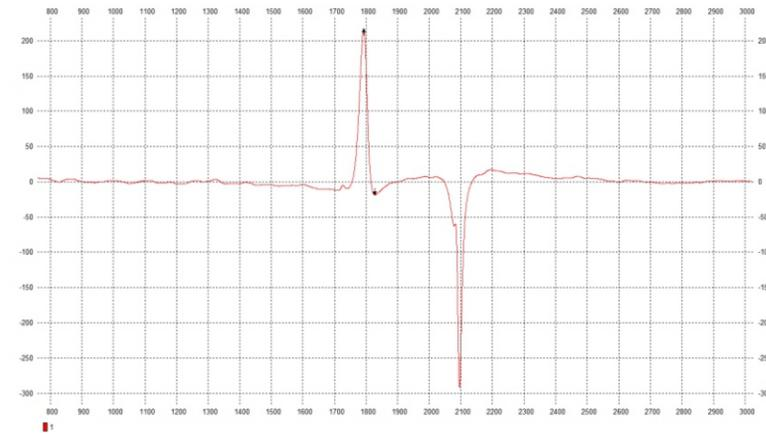
Magnetic profile of ferrous debris field **7482**, measuring 237 nT
