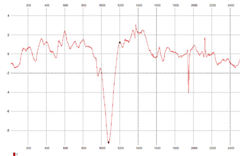
Magnetic profile of wreck 7477, measuring 11 nT
