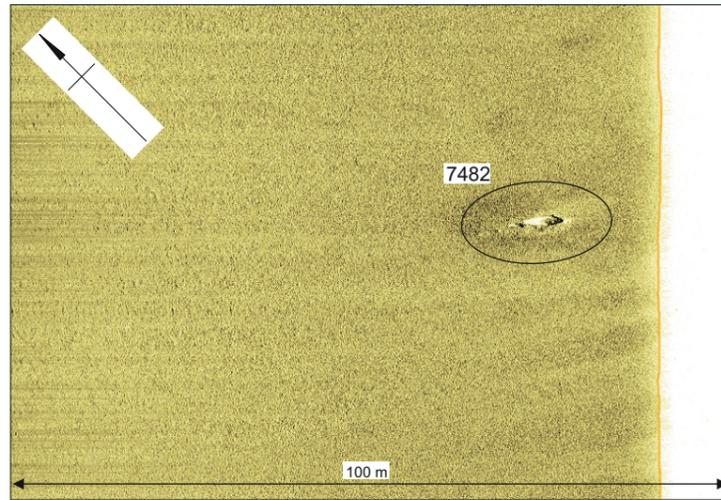
Sidescan sonar waterfall image of ferrous debris field **7482**, 10.0 x 10.0 x 1.1 m
