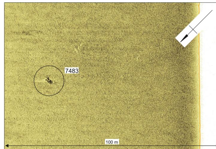
Sidescan sonar waterfall image of dark reflector **7483**, 9.9 x 4.0 x 0.7 m
