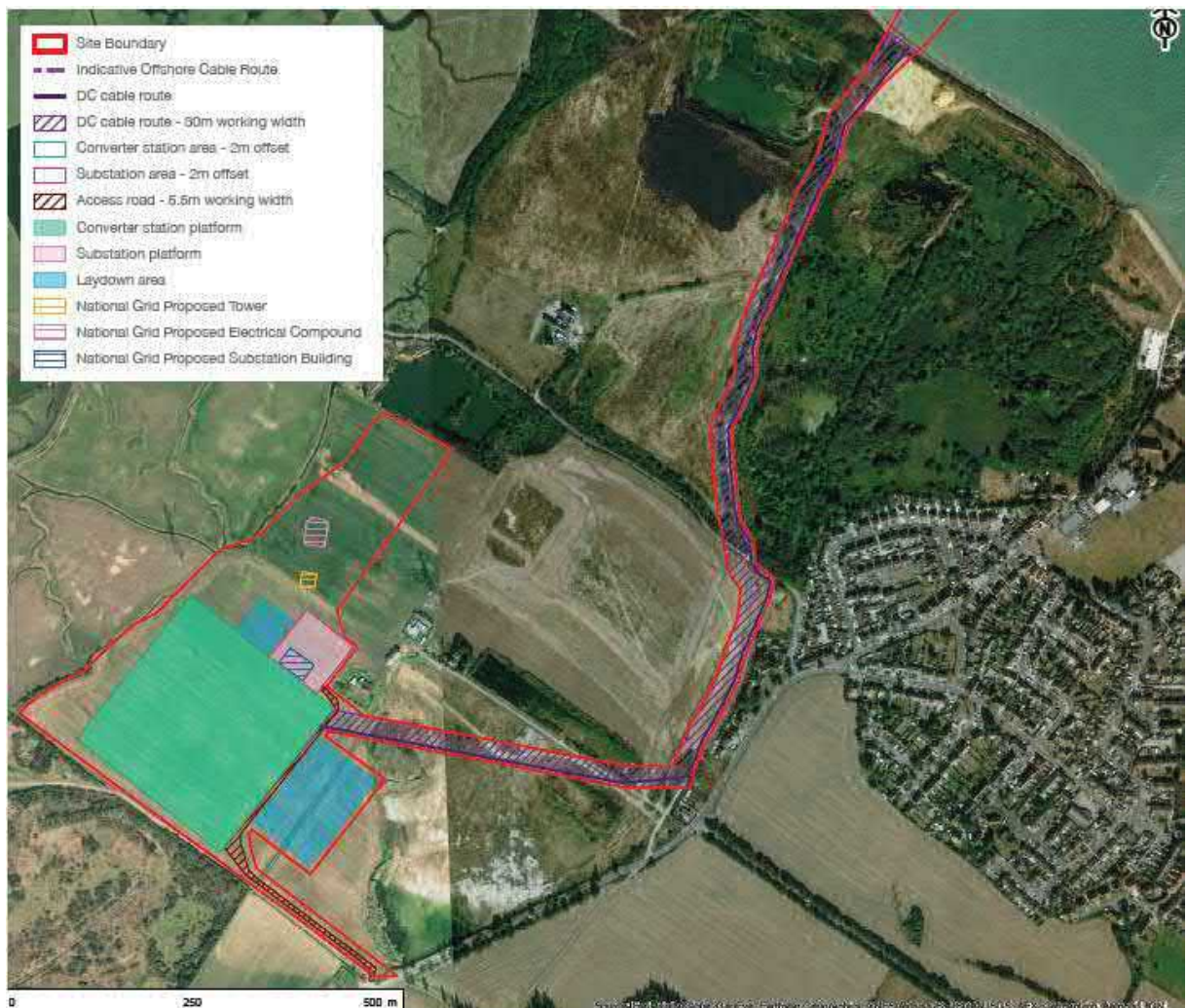
A satellite image depicting the GB onshore elements at the site on the Isle of Grain.
