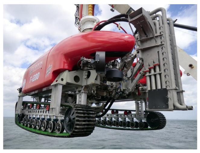
Modern ROV water jetters can bury cables to a typical depth of 2-3 metres, and the latest models even up to 5m when using a cable depressor.
