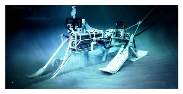
For burial to depths considerably deeper than 2-3metres below seafloor, for example, up to 10meters into sands, in areas closer to shore, the Vertical Injector (VI) technique is recommended. Machines like the one shown in Figure 7-5 are designed for SLB operations.
