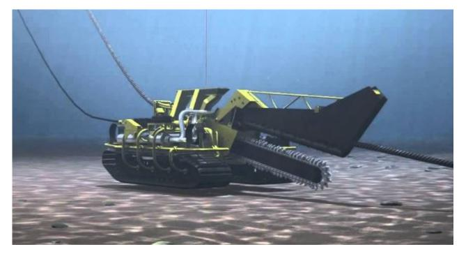
When using this method, the trench should remain as narrow as possible and the trench is typically filled in by the natural movement of the seabed materials. In hard soils where rock trenching is necessary, a reduced burial depth is typically acceptable considering reduced anchor and trawler penetrations into the seabed.
