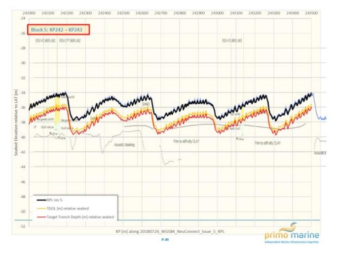
The Table 12-3 below provides a detailed summary of the segmentation of the UK Sector route based on Shallow Geology, with the depth of interest being the Target Trench Depth (TTD) profile (see red line in Figure 12-3, the orange line represents the TDOL profile).
