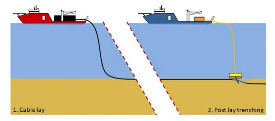
It should be noted that SLB is not necessarily always faster than surface laying the cable in a first pass, followed by post-lay burial (PLB) in a second pass (often with a different vessel) – see Figure 7-3.
