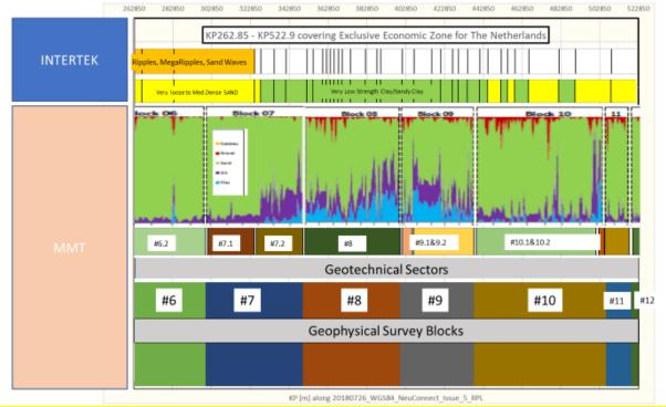
Comment: Moderate to Good correlation between geotechnical segmentation by MMT and sediment type segmentation by Intertek.
