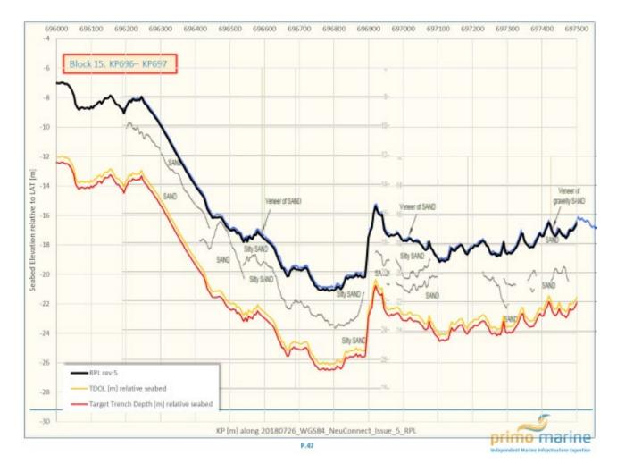
The Table 14-3 below provides a detailed summary of the segmentation of the GERMANY Sector route based on Shallow Geology, with the depth of interest being the Target Trench Depth (TTD) profile (see red line in Figure 14-3, with the orange line representing the TDOL profile).
