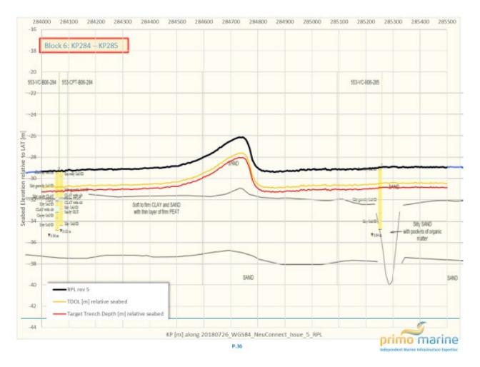
The Table 13-3 below provides a detailed summary of the segmentation of the NETHERLANDS Sector route based on Shallow Geology, with the depth of interest being the Target Trench Depth (TTD) profile (see red line in Figure 13-3, with the orange line representing the TDOL profile).
