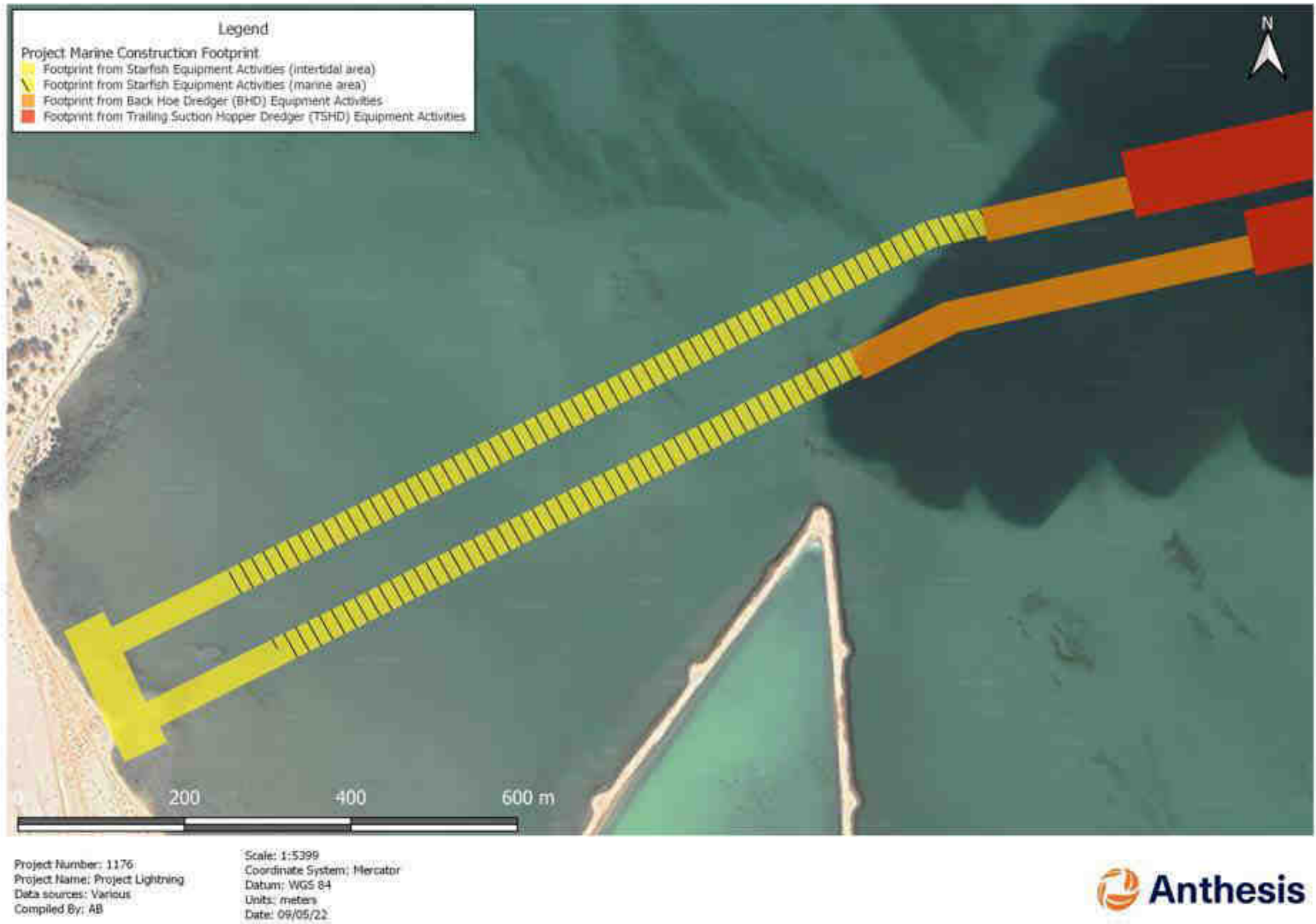
Figure 4-67: Detailed marine construction footprint for Mirfa nearshore area (Route 1) (KP 0.000 to KP 1.500)
