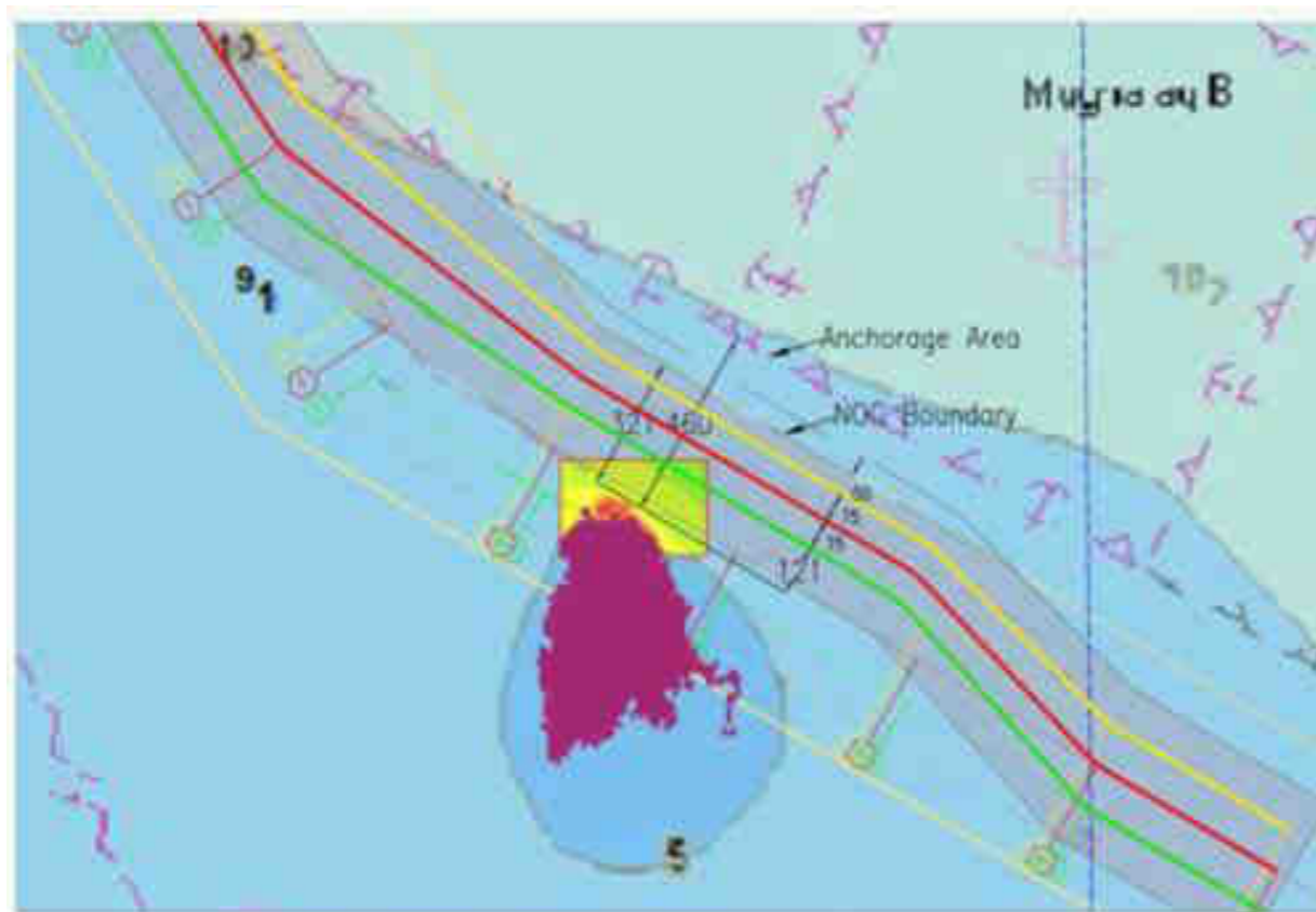
Figure 6-9: Route 2 alignment changes to avoid the patch reef area and the Mugharraq anchorage areas
