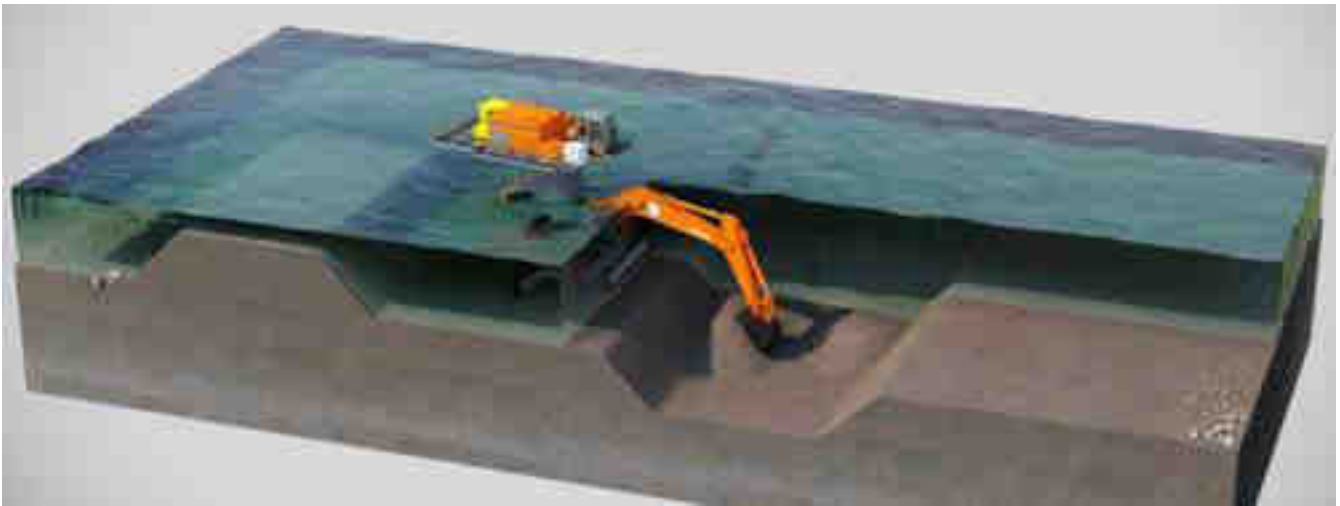
Figure 4-74: Starfish excavating pre-trench design
