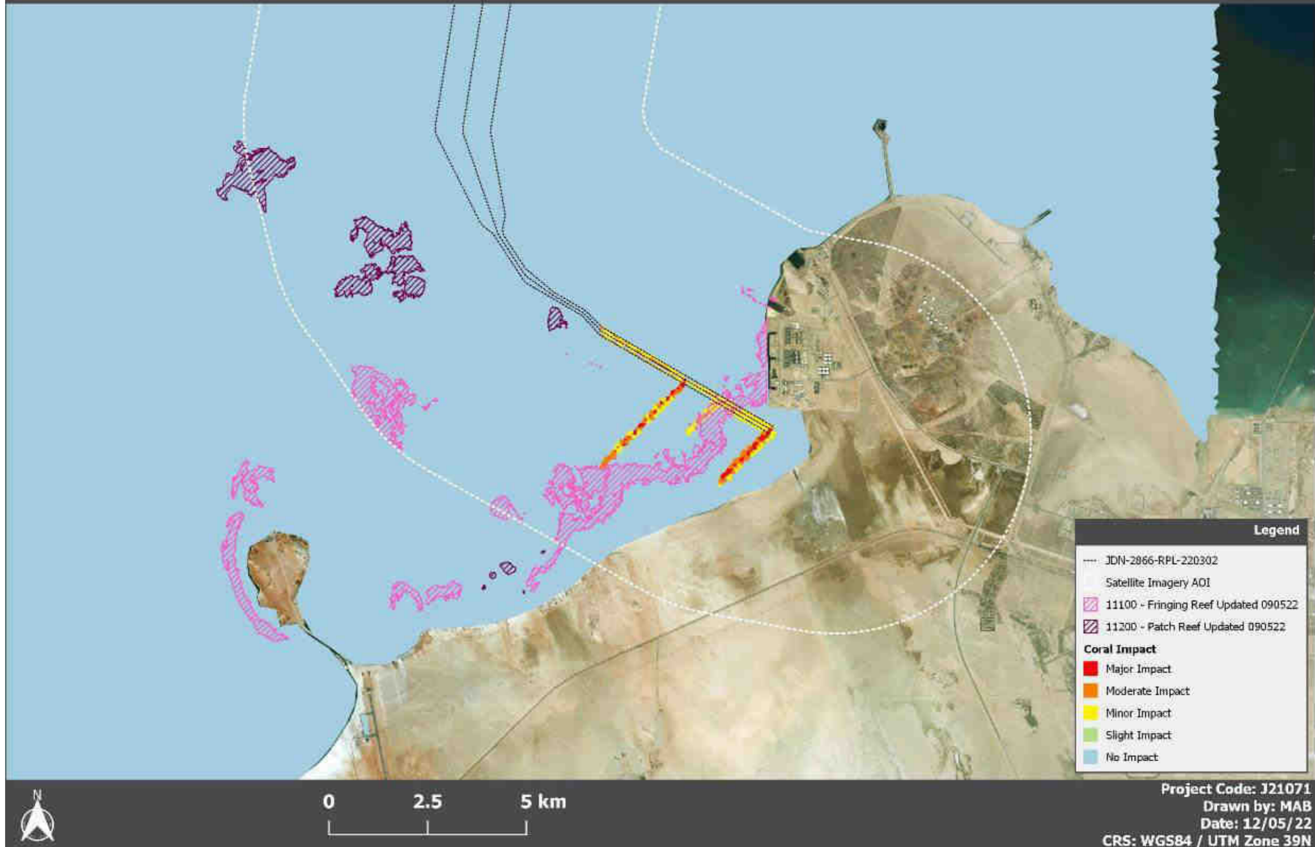
Figure 5-47: Impact of average fortnightly sediment deposition on coral reef habitats along Route 2
