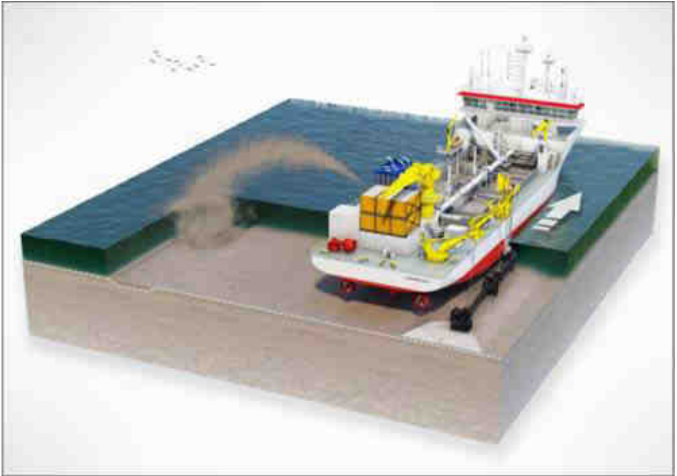
Figure 4-83: TSHD backfilling via spraying
