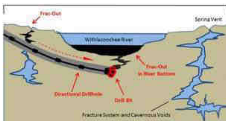
Figure 6-11: Illustration of frac-out
