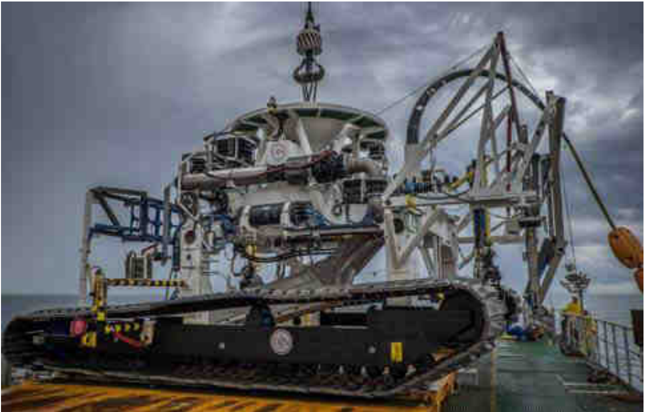
Figure 4-89: UTV 1200 post-lay trencher
