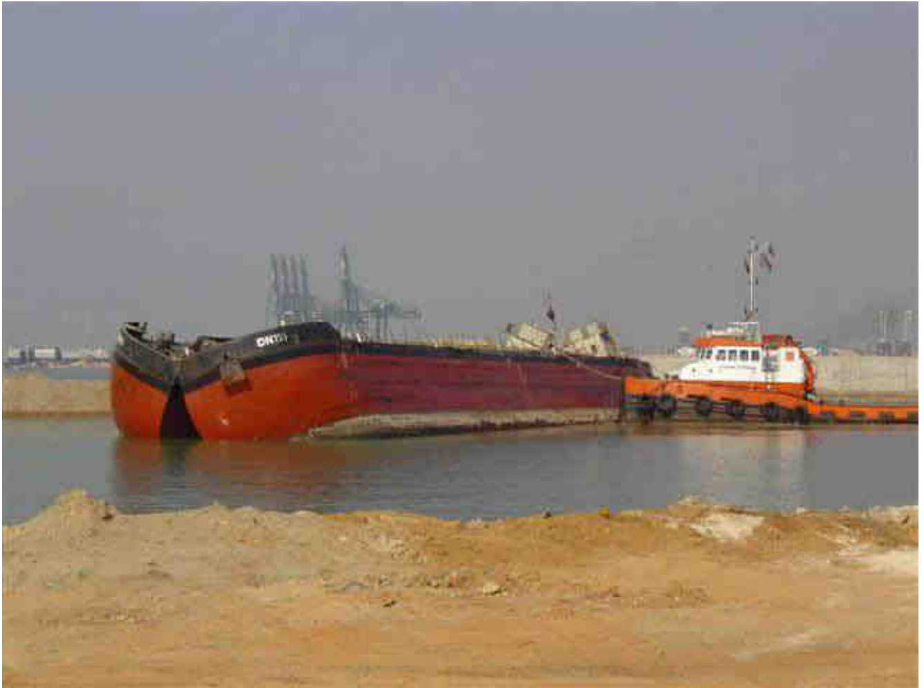
Figure 4-78: Split Hopper Barge (SHB)
