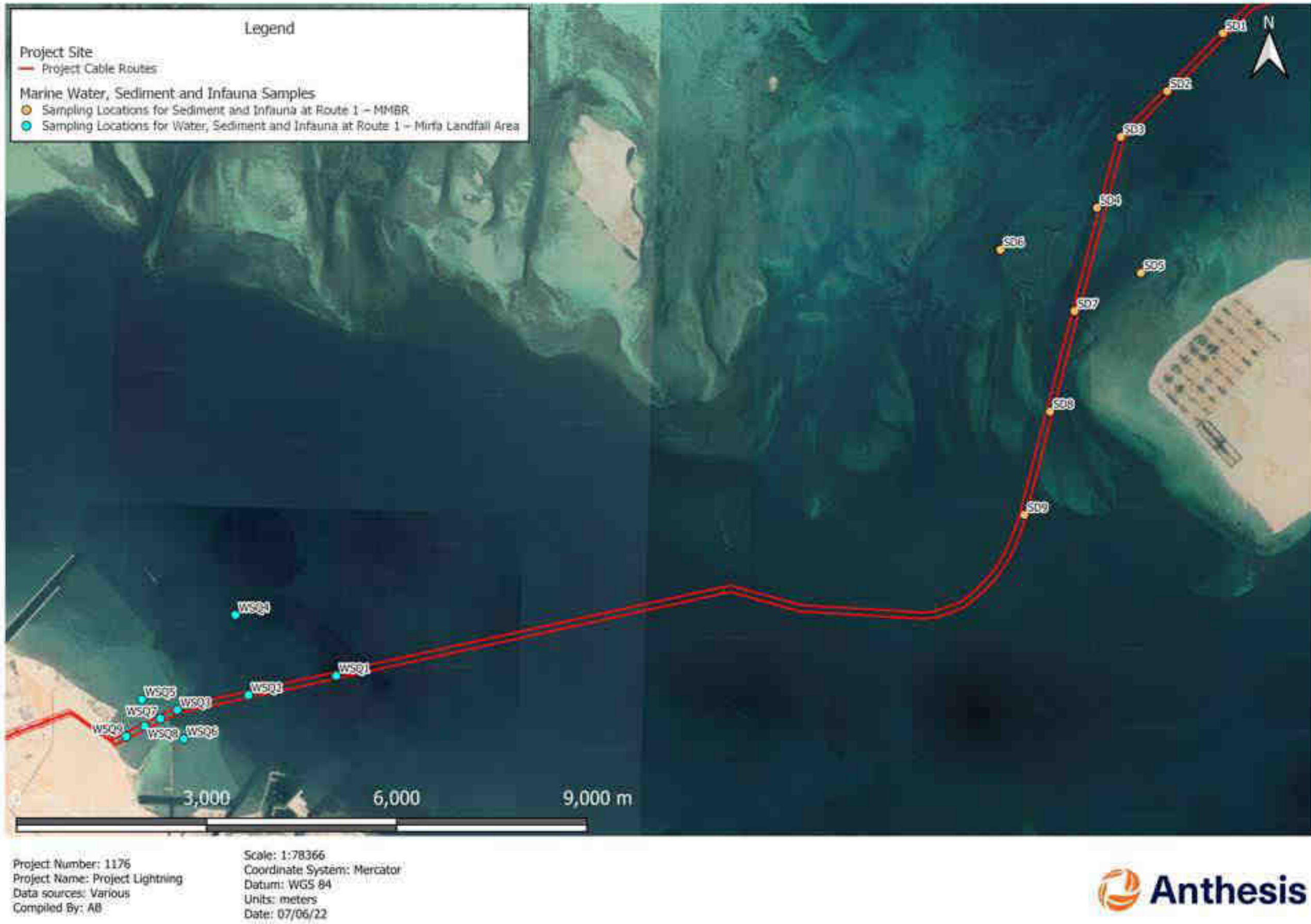
Figure 5-11: Water and sediment quality sampling locations along Route 1 – Mirfa Landfall and Mirfa Nearshore Area within and near MMBR
