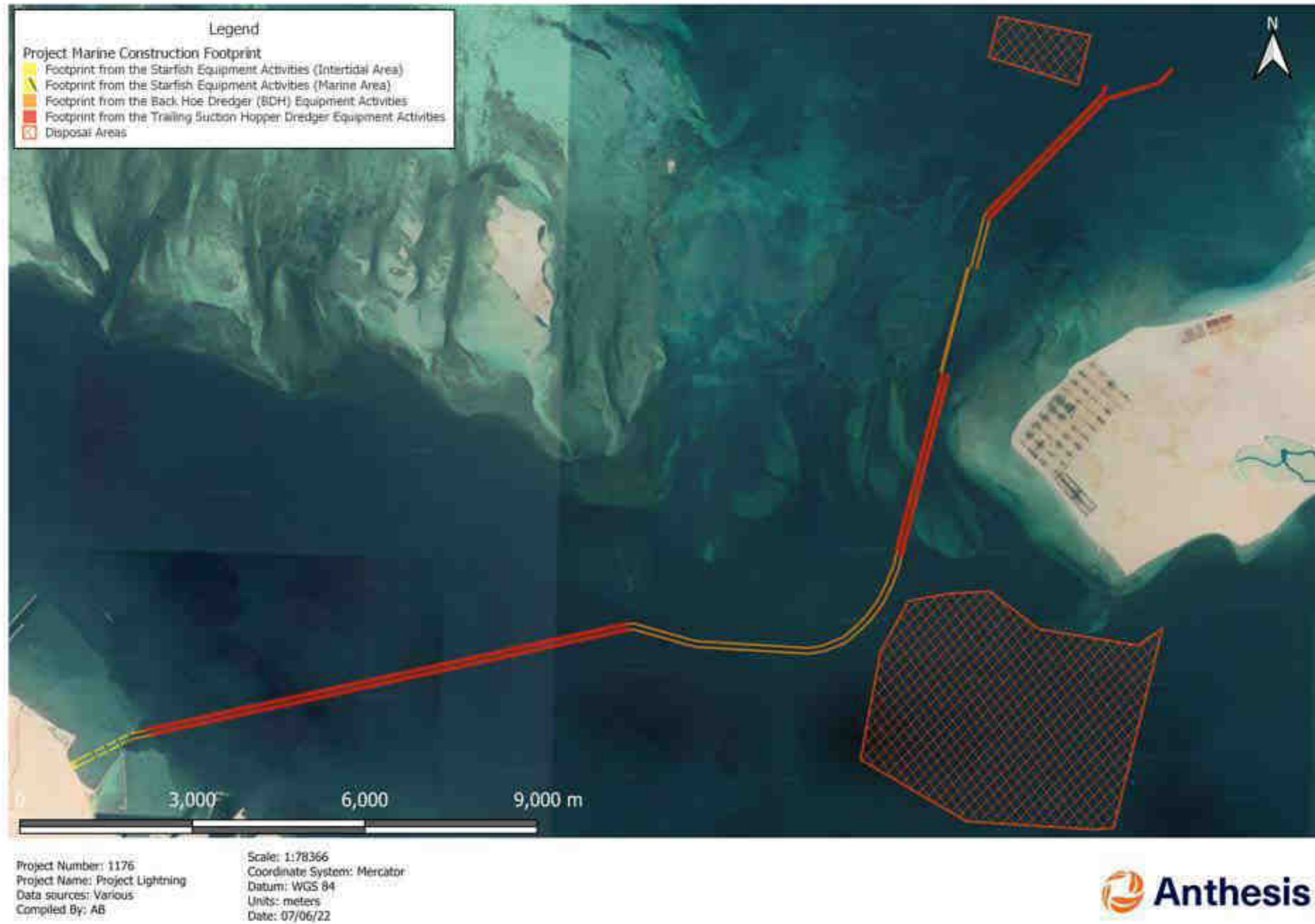
Figure 4-66: Overview of the marine construction footprint for Mirfa nearshore area (Route 1) (with the disposal areas) (KP 0.000 to KP 26.000)
