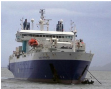
Cable Laying Vessel (source : Nathan Sandel)
